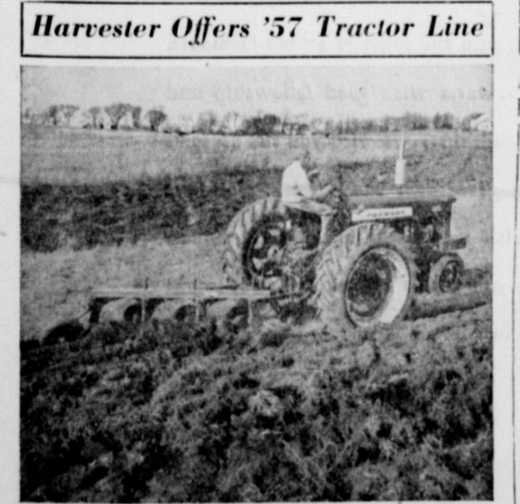
This is the Farmall 450 in the new 1957 farm tractor line now being shown by International Harvester dealers everywhere. The "450" is shown here with the new Fast-Hitch with Traction Control pulling the new McCormick four-bottom plow.
