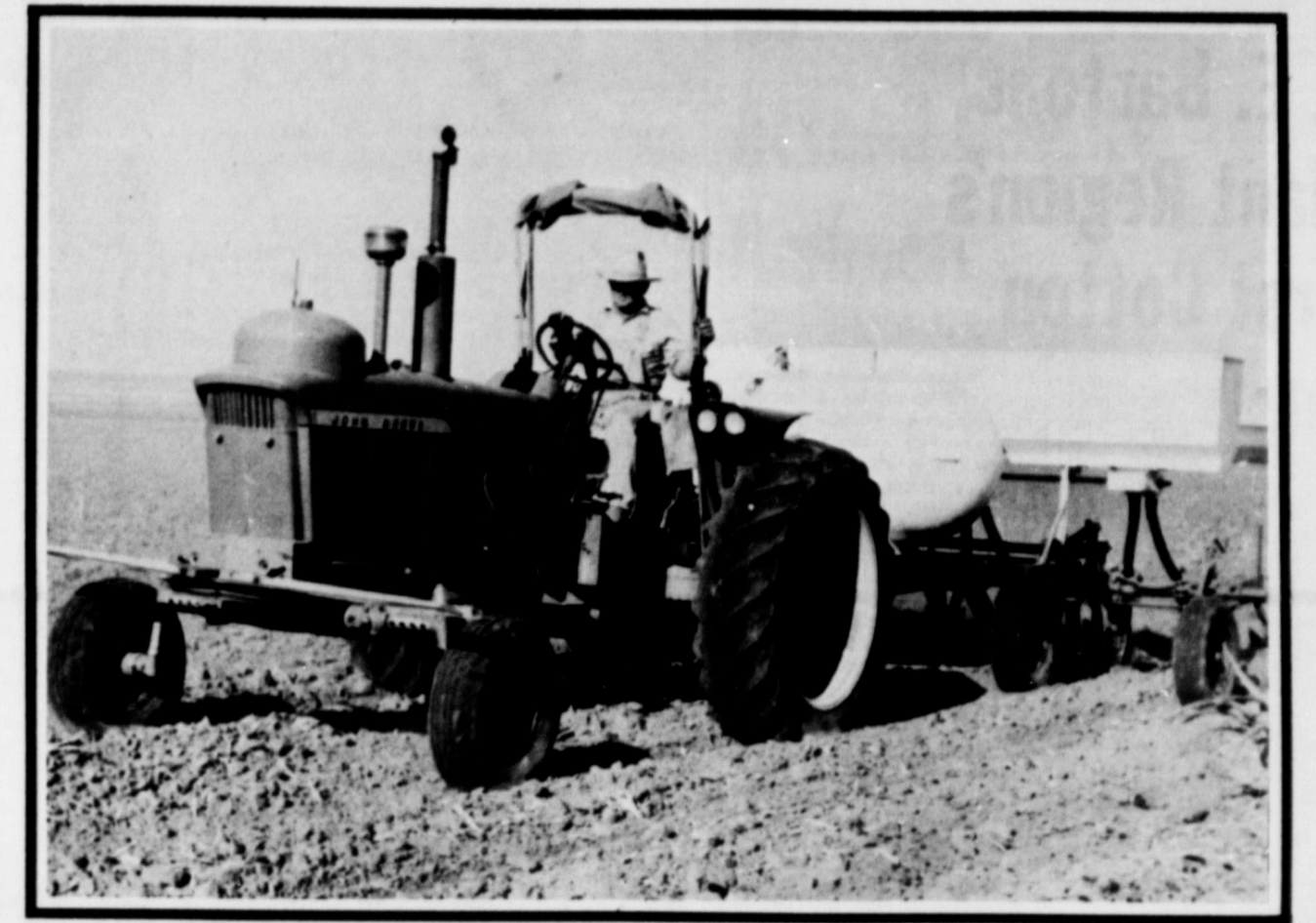
PICTURED ABOVE IS TROY BLACKBURN USING THE NEW DUAL TEST RIG, BANDING IN DRY FERTILIZER AND APPLYING ANHYDROUS AMMONIA AT THE SAME TIME.
