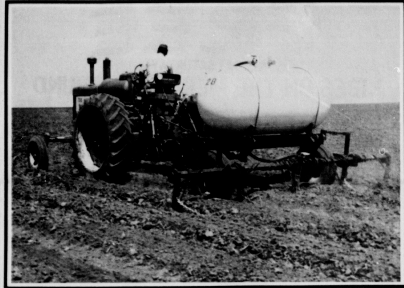
PICTURED ABOVE IS A FOUR ROW ANHYDROUS AMMONIA PRE PLANT RIG WITH A 350 GAL. SUPPLY TANK.
