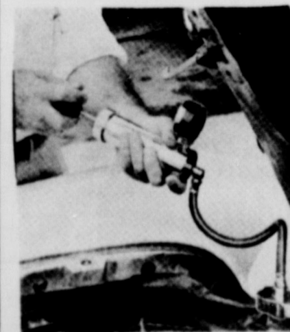
Pumping up pressure in the cooling system.
