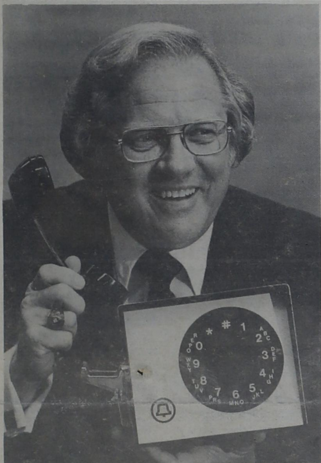
TELECOMMUNICATIONS WIZARDY —Southwestern Bell's science demonstrator Bill Haehnel displays a telephone that doesn't have to be dialed. The device, which responds to verbal commands, is one of the innovations from Bell Labs featured in Haehnel's show, "An Adventure in Communications."
