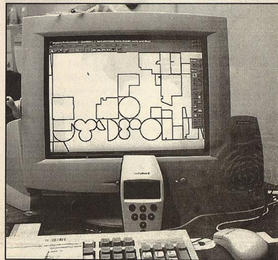
Electronic wizardry being used in weevil war includes this Geo Explorer II, between keyboard and computer monitor, down loading data from orbiting satellites for field mapping
