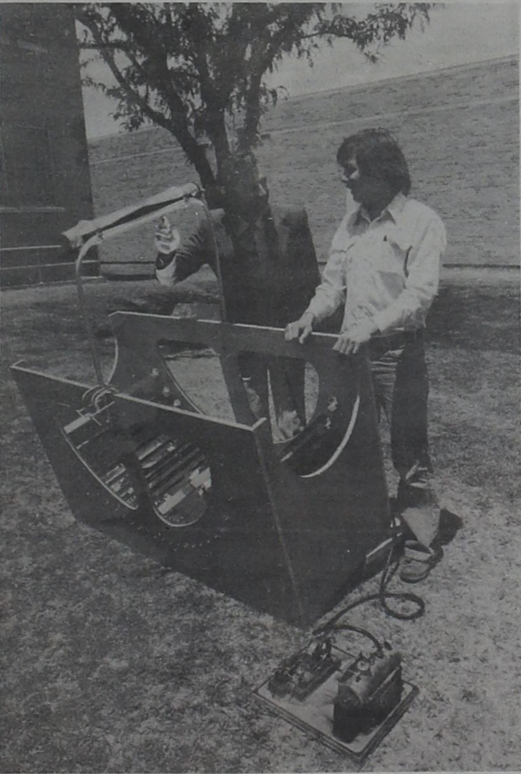
SOLAR STEAM ENGINE —Dr. Norman Sheridan, left, visiting professor of mechanical engineering at Texas Tech, discusses a solar-powered steam engine with student Henry Kight. Kight built the project as an assignment for a solar energy seminar taught by Sheridan. A series of mirrors focus light on a water-filled heat converter. The heat and water produce steam, which is transferred through rubber tubing to the engine. (Tech Photo)
