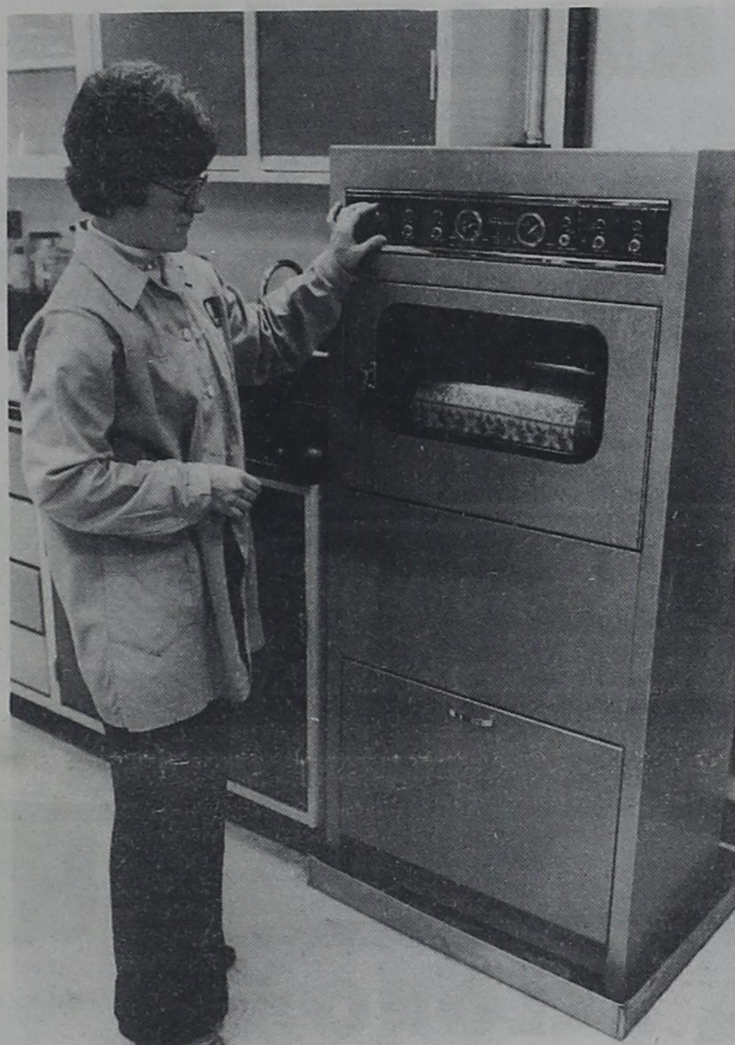
"LAUNDRI-LAB TESTER"—Lab technician Norma Keyes of the Cotton Incorporated research center at Raleigh, N.C., adjusts the controls of the new machine, developed through cotton producer research, to help cotton customers meet government flame retardant regulations.
