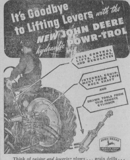
Think of raising and lowering plows . . . grain drills . . . cultivators . . . mowers . . . combines . . . corn pickers-of angling and straightening disk harrows-of instantly changing working angle, depth or height without stopping or slowing down-all at a touch on a convenient lever!
