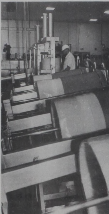
AT LEFT, Prentise Burkhart fills the 500-pound barrels with stirred curd cheddar cheese, which is then pressed, here by John Kidd.
