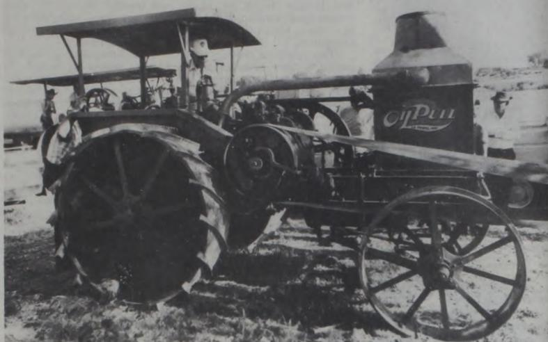
**THE MODEL H,16-30 Advance Rumely Oil Pull Tractor** appeared in 1919. The two-cylinder engine operated at 530 rpm and developed a 4,674-pound drawbar pull and cranked out 32.52 brake horsepower. Production ended in 1924, with a total of 56,647 oil pulls being built in 14 different models.
