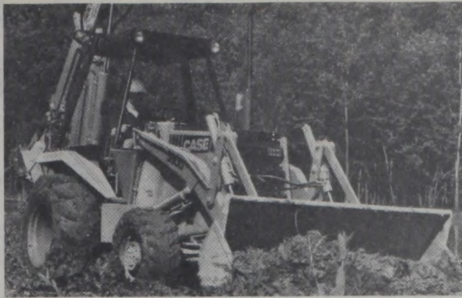
Backhoe Option - Mechanical four-wheel drive is now available as a factory installed option for the Case 580D backhoe-loader, according to J.I. Case Co. Case Power and Equipment, Gainesville, is the only Case dealer in the area, and the new option provides the only four-wheel drive backhoe in the industry.
