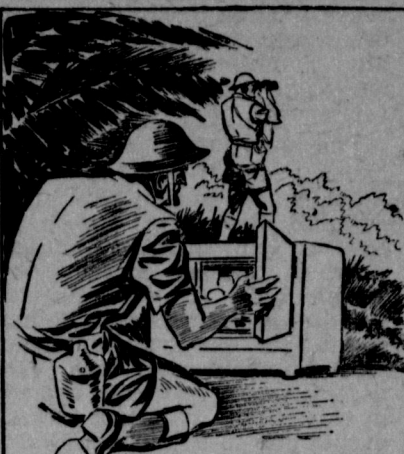
A RECENT DEVELOPMENT IS A PORTABLE REFRIGERATOR WITH A MOTOR THAT CAN BE RUN BY EITHER GASOLINE OR ELECTRICITY. IT CAN BE USED ANYWHERE—ON SHIP, OVERSEAS, AND IN ISOLATED OUTPOSTS.
