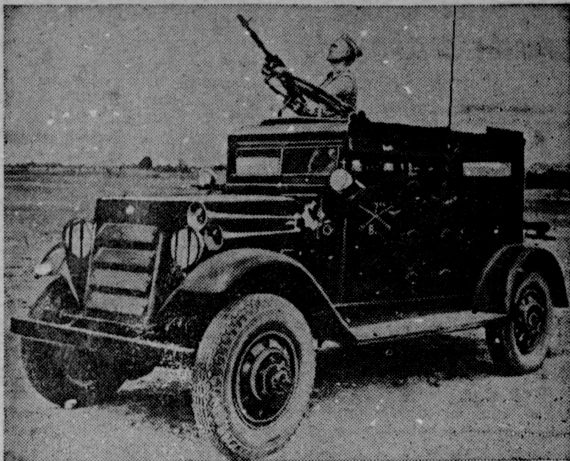
Here is one of the combat cars of the mechanized force of the United States army participating in extensive maneuvers in the Middle West. In time these cars, capable of great speed and heavily armed, will displace cavalry in war. All the cars are equipped with two-way radio for keeping in constant touch. The "cavalryman" shown here is operating an anti-aircraft gun.
