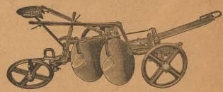
They weigh less, run lighter and do better work. They are simpler in construction, with to get out of fix. They are strong and rigid. Their frames are low down, so that they run Their leverf are in reach of the driver. The tongue can be adjusted to any position. The disare made of chilled iron and are oiled by means of compression grease cups. The rear end of can be raised or lowered as occasion may require. Large bolts are used throughout.
