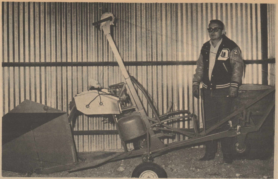
MAN AND HIS MACHINE—Dick Morrison poses beside his nearly completed gyrocopter in Sunnyside. Morrison, manager of Morrison Gin, says the craft will do 70 miles an hour with a 70 horsepower motor, and will land at 20 miles an hour.
