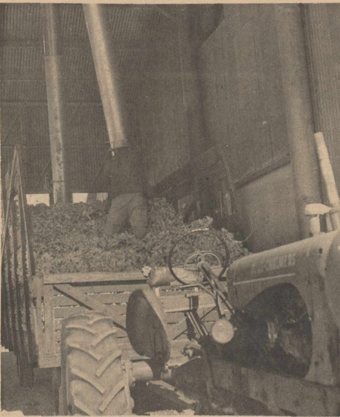
THE COTTON GOES IN HERE -- Area gins are going full blast right now trying to catch up with the rapidly moving area harvest. And it all starts right here, where suction tubes are used to move the crop from field trailers into the gin.
