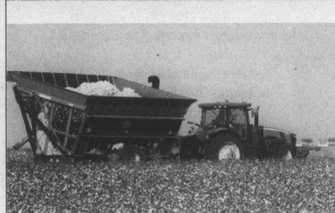
It's a process ... It's a lengthy process to harvest the cotton acreage, from gathering the cotton with a cotton stripper, dumping it into a boll buggy, and then forming it into modules, before gins can then process it into bales. (LCN PHOTOS by Gary Jones)
