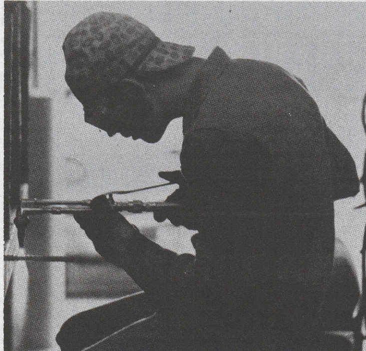
Welding Dept. — Lydell Ashley shown here using the acetylene touch torch.
