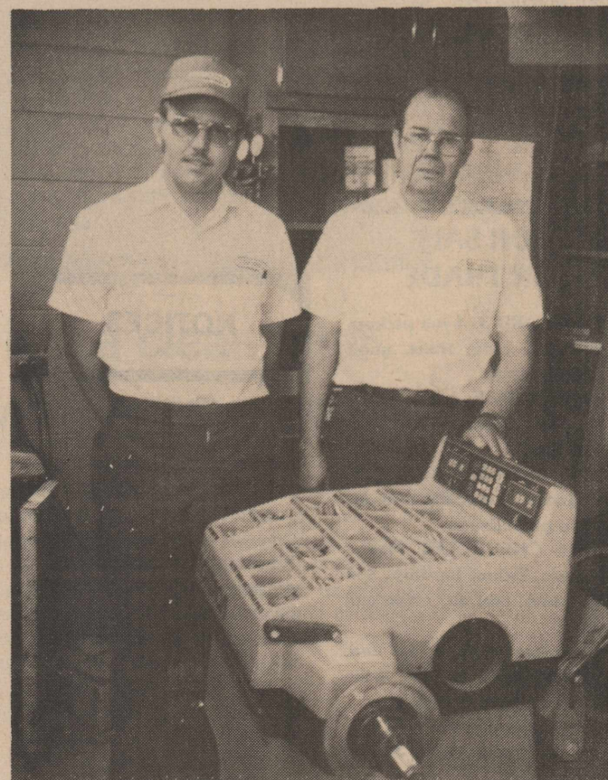
THE VERY LATEST equipment now available at Marion Conoco Station is this new microprocessor precision wheel balancer. Owners, from left, Roland and Joe Marion explained that the Nortron computer spin balancer balances both sides of a tire separately and can accommodate both autos and light trucks.
