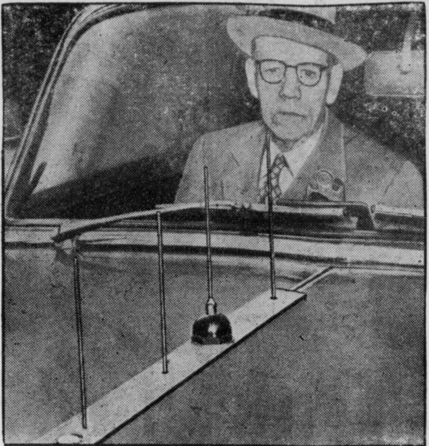
ROBOT GUARDIAN—Emergency vehicle's broadcasting antenna is examined by Police Chief Jeremia O'Connell, of St. Louis, Mo. Vehicle equipped with the device projects a radio beam ahead of itself. Beam energizes special devices atop signals, setting their indications to "danger" and actuating special warning lights.
