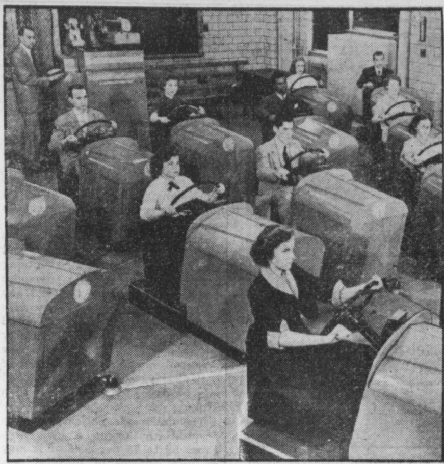
Brooklyn High School students study ins and outs of safe driving in behind-the-wheel classes. Using Aetna Drive-trainers, the students "drive" over highways shown on a movie screen. Their reactions are shown in detail on the instructor's panel at left.
