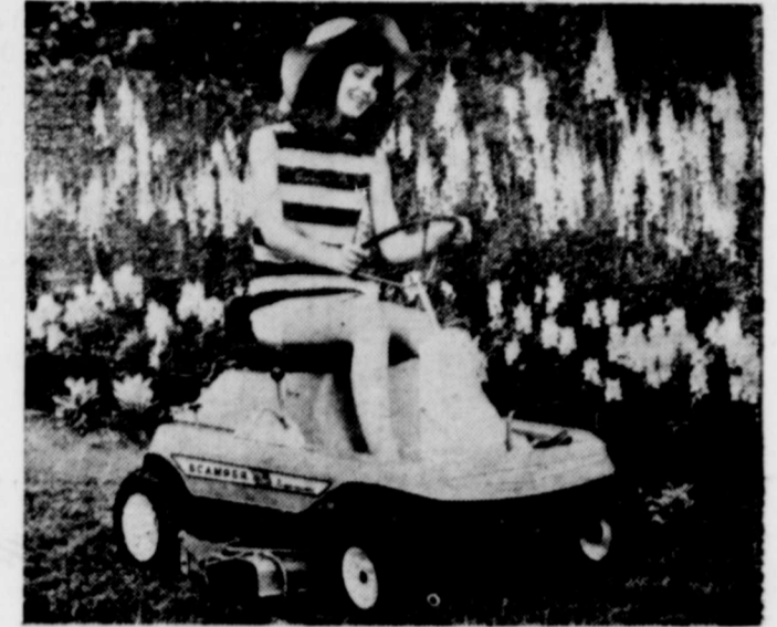
Allis-Chalmers added this riding mower to its lawn and garden equipment line. The 7 horsepower mower, called the "Scamper," has an automatic drive transmission for on-the-go shifting. The mower cuts a 36-inch swath with free floating action to prevent scuffing and gouging.
