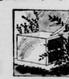
Trim shrubbery: The outdoor unit needs free air circulation. Help it maintain full efficiency and keep operating costs down by trimming nearby shrubbery and by checking to make sure compressor coils are clean.
