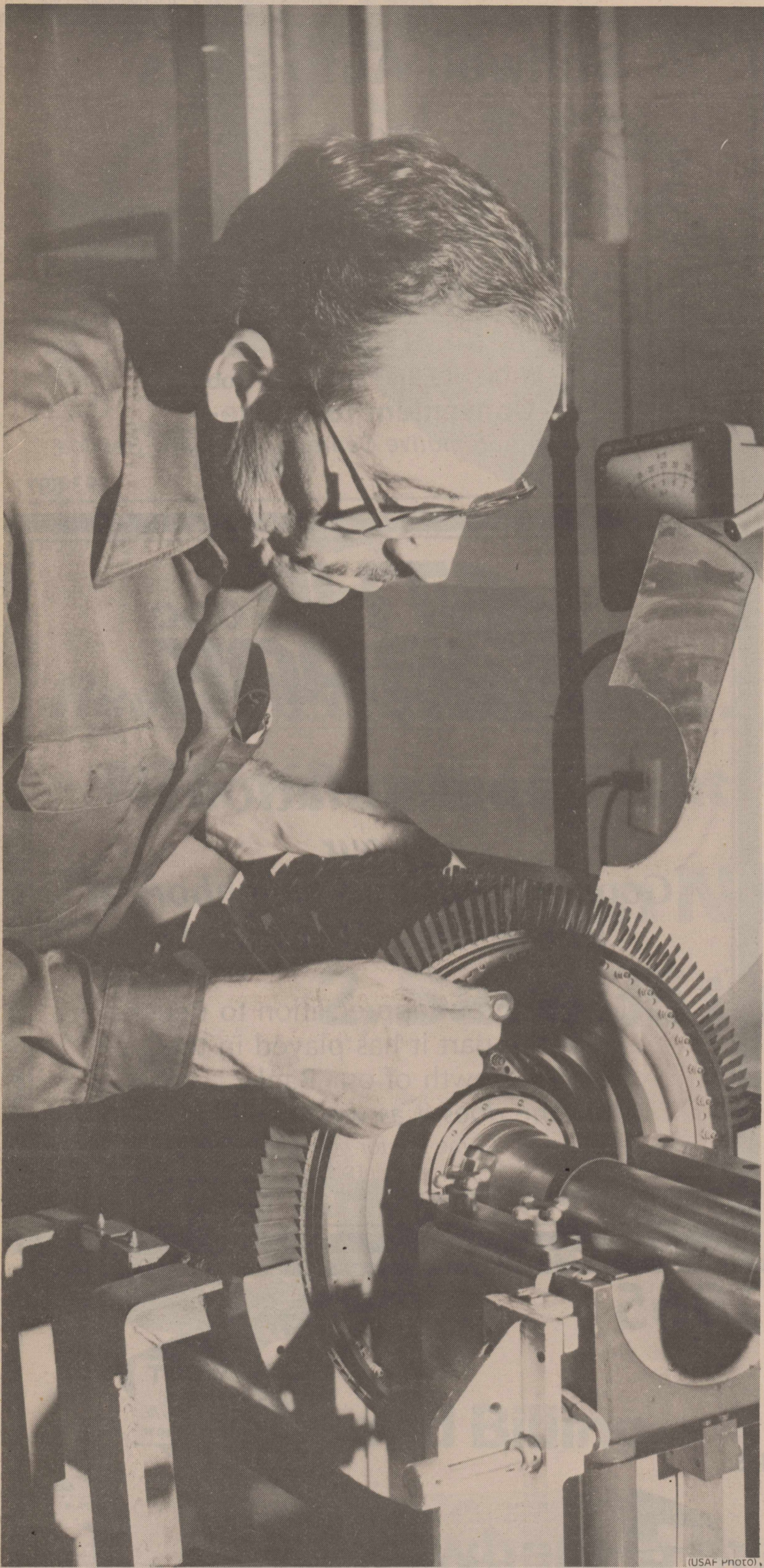
A civilian employee at Reese adjusts the delicate fan blades in a jet engine. One of the reasons that the aircraft here have flown here for so long is the continued maintenance program—which stresses attention to detail.
