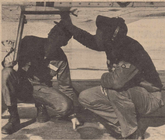
ASSISTANCE — Airman First Class Donald Lemke, an electrician from field maintenance, inspects and adjusts an inverter valve on a T-38 Talon after AB Warren Moore, organizational maintenance crew chief, requested specialist assistance from the maintenance scheduling section. Airman Lemke and other specialists are on constant alert to assist flightline crews in fast repair of training aircraft.
