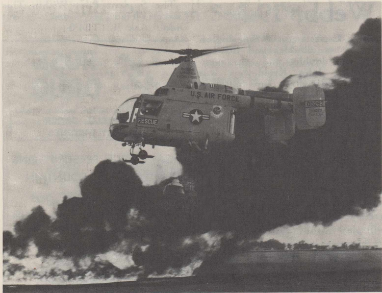
FIRE-FIGHTER —An HH43B helicopter used in Reese search and rescue work moves in on a blazing fire to help firemen extinguish it. The propellers turn back heat, smoke and flame and permit the firemen to reach any crash victims quickly to bring them out for speeding to a hospital.
