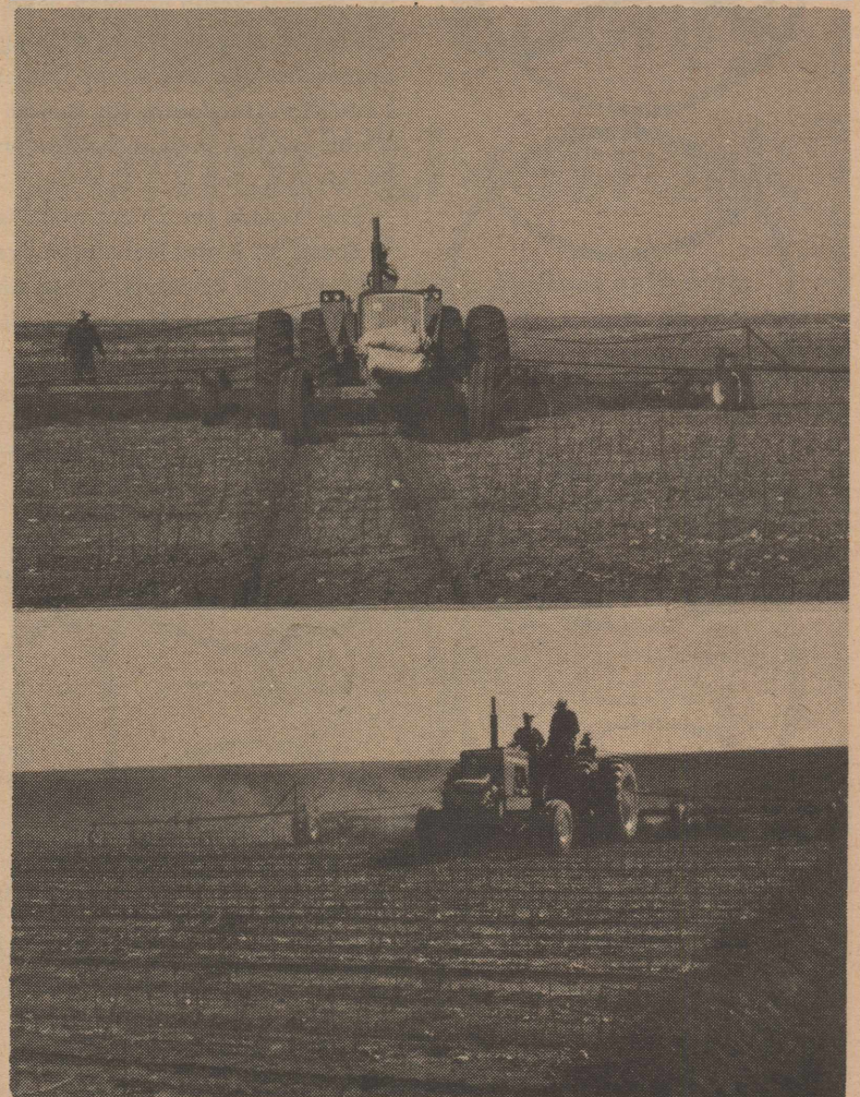
THE 12 ROW LISTER IS BEING PULLED BY A 220 ALLIS CHALMERS TRACTOR. IT IS WORKING ON THE J.D. NIX FARM IN THE EAST PART OF GAINES COUNTY. IT WAS TRAVELING AT 5 MPH WHEN THE LOWER PICTURE WAS TAKEN.
