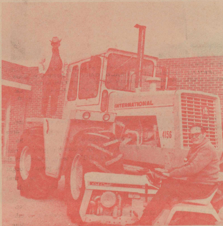
How's this for a Christmas present? Albert McGuire admits this 4156 International tractor is a gift from Albert to Albert. Riding a Cub Cadet in the foreground is Elbert Medlin from LMH Truck and Tractor, Inc. The huge tractor has a draw bar estimated at 125 horses, 140 horses PTO (power take off). The industrial tractor has a four wheel drive and will be used in the farming operation on the McGuire farms. It will easily handle a 12 row planter or a large five disc Baker plow. It has power brakes and power steering.
