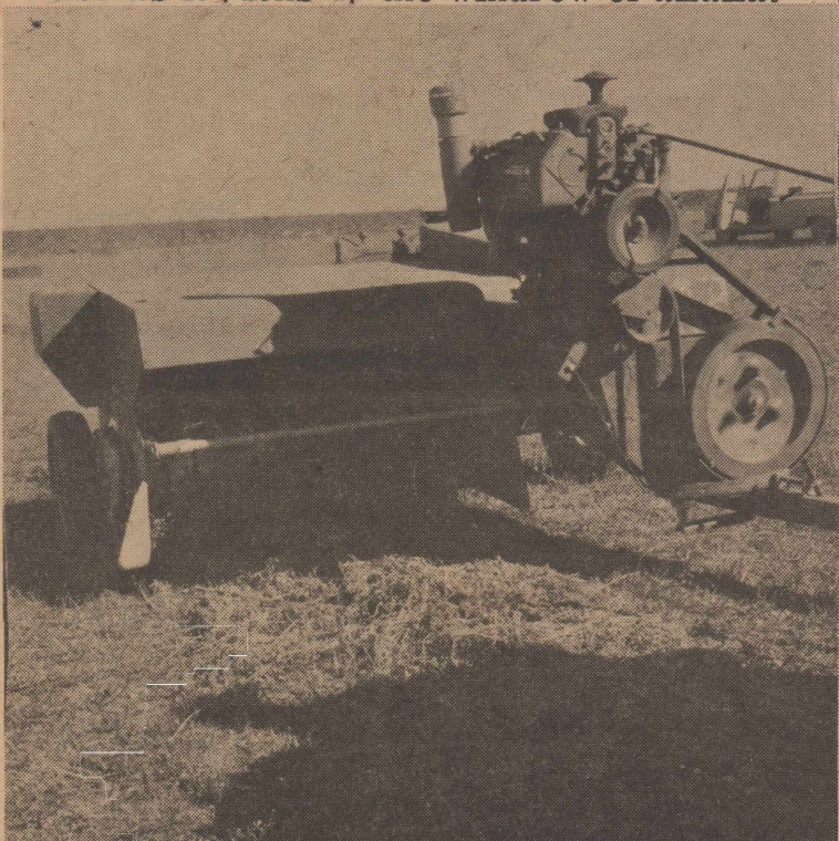
Maybe some of us can remember the days when 200 bales was a good day's run. This motor driven machine will bale that much in an hour.
