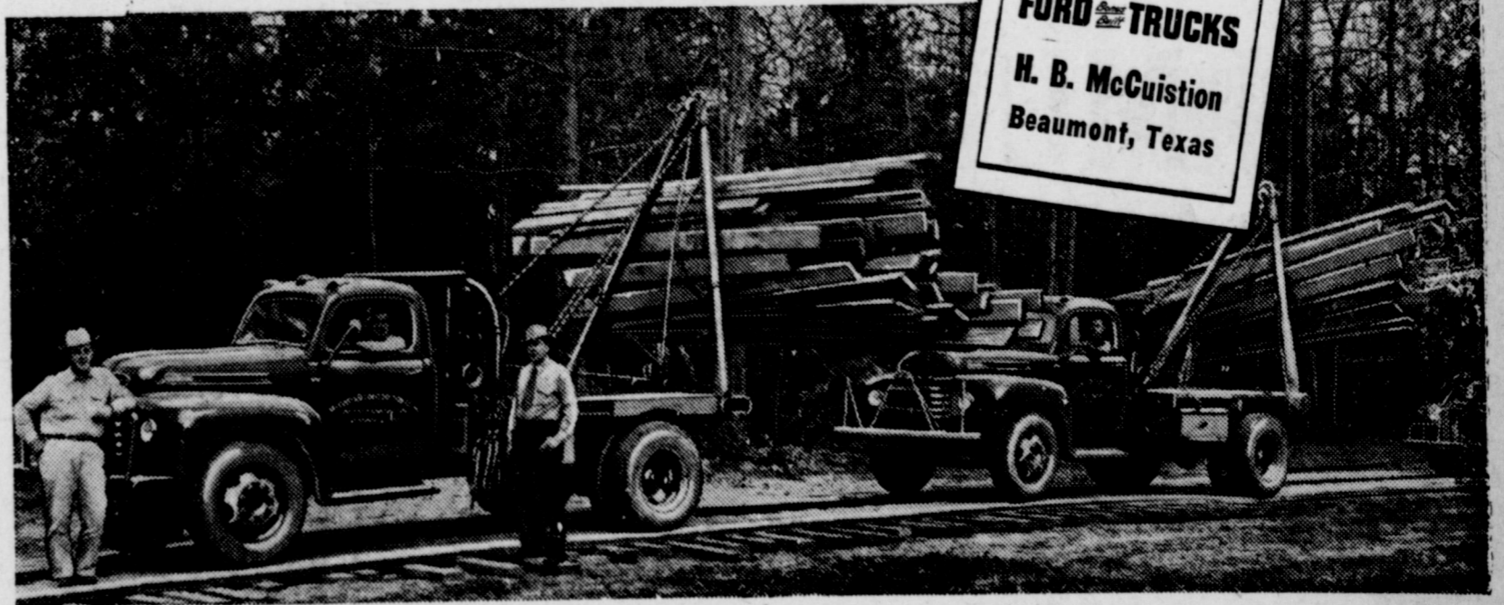
Ford Model F-7 Big Job shown has Gross Vehicle Weight rating of 18,000 lbs., Gross Combination Weight rating of 35,000 lbs. as a tractor.
