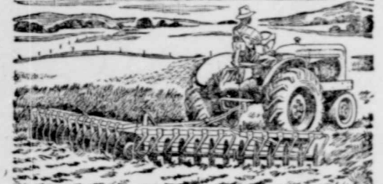
No. 15 Series Single Action Disc Harrow — designed to cover large areas quickly. 15-foot size quickly "telescopes" to go through 10-foot gate without lifting or exposing dangerous discs.
