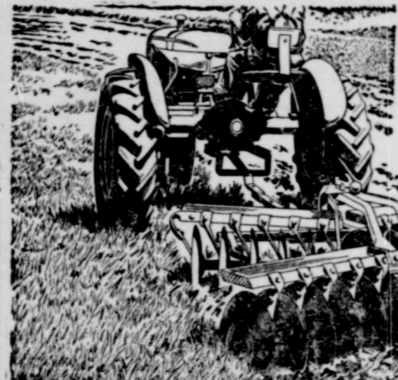
No. 9 Series Tandem Disc Harrow — for average working conditions. Square, welded, steel tubing frame double the strength of ordinary angle iron.
