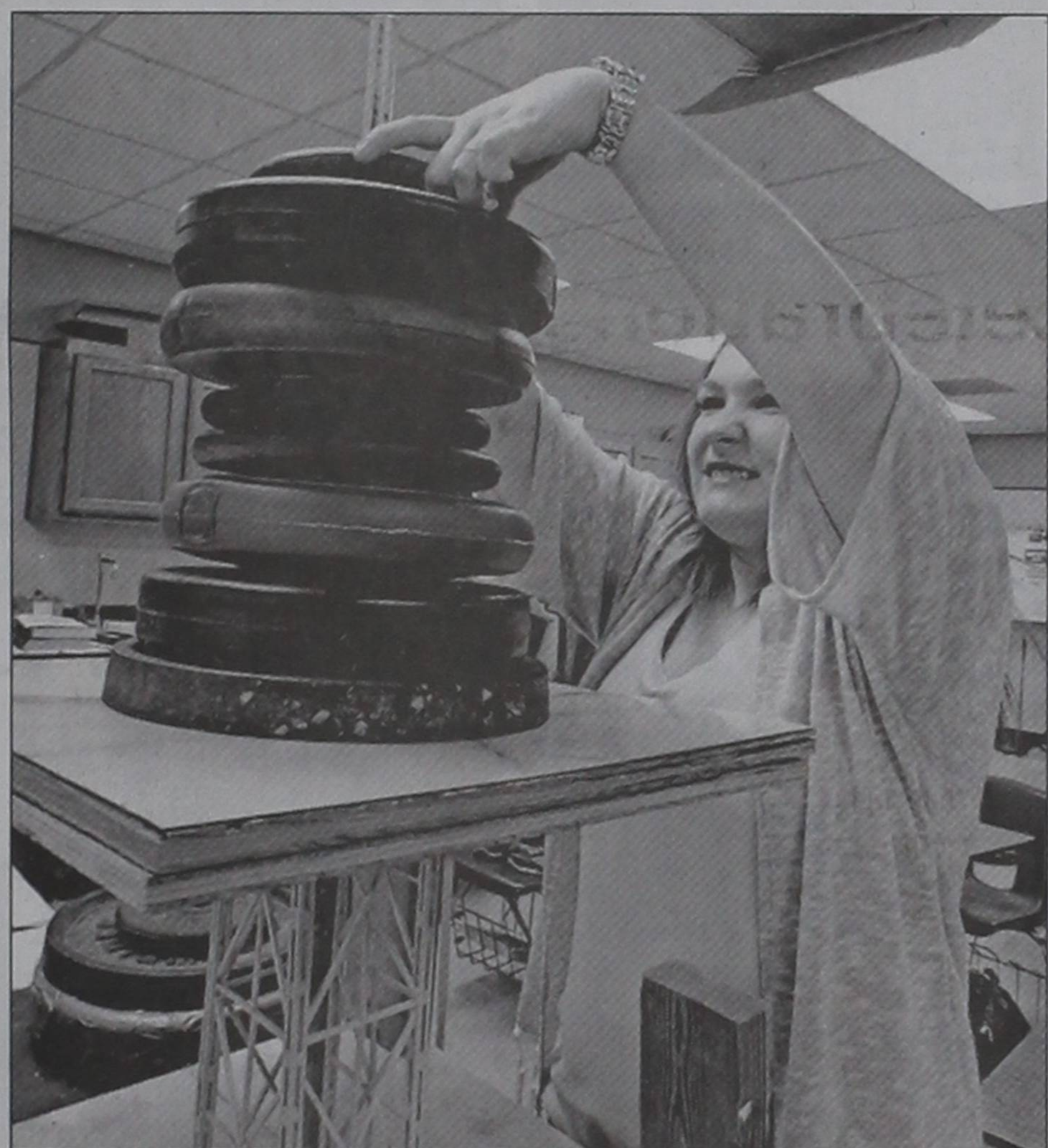
The CHS Physics class built balsa wood towers for their annual competition. This years winners were Shelby Baxter (pictured) and Karlee Adams, who built a tower only weighing only 1.1 ounce that held 162 pounds of weight before it failed.
