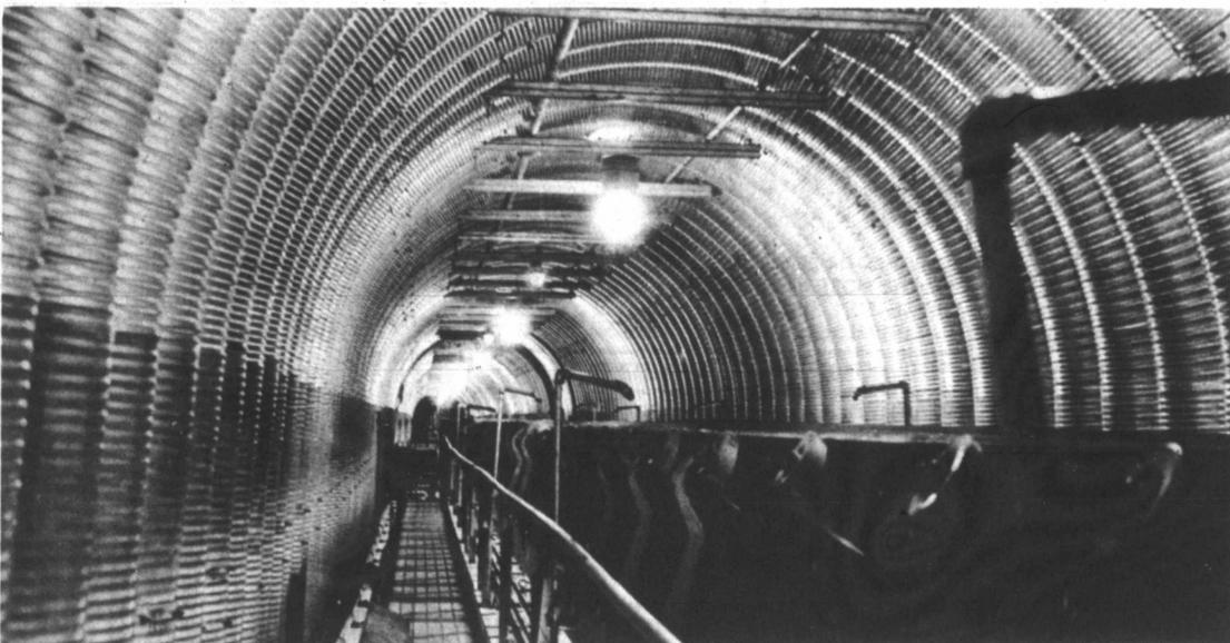
**INSIDE THE CONVEYOR** which transports the coal from the four underground receiving hoppers to the stacker. From here the coal is conveyed to the crusher where it is reduced to a size acceptable for firing. It is then conveyed to surge bins, which are covered to prevent dust emission.
