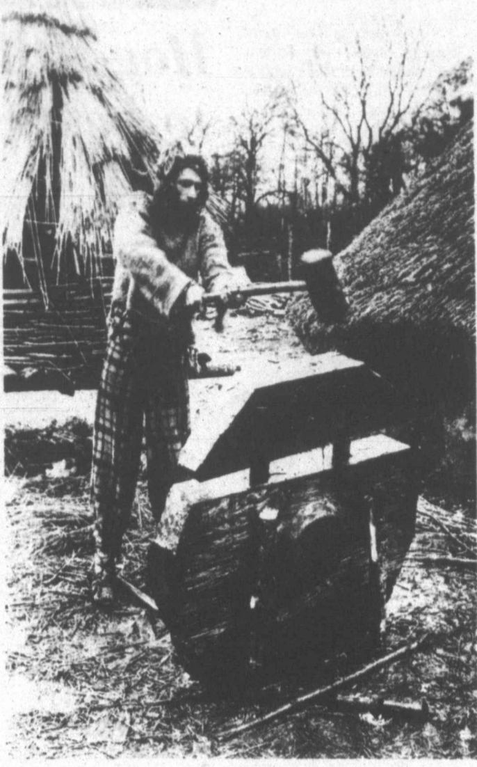
Peter Little makes an oak cartwheel with handmade tools.
