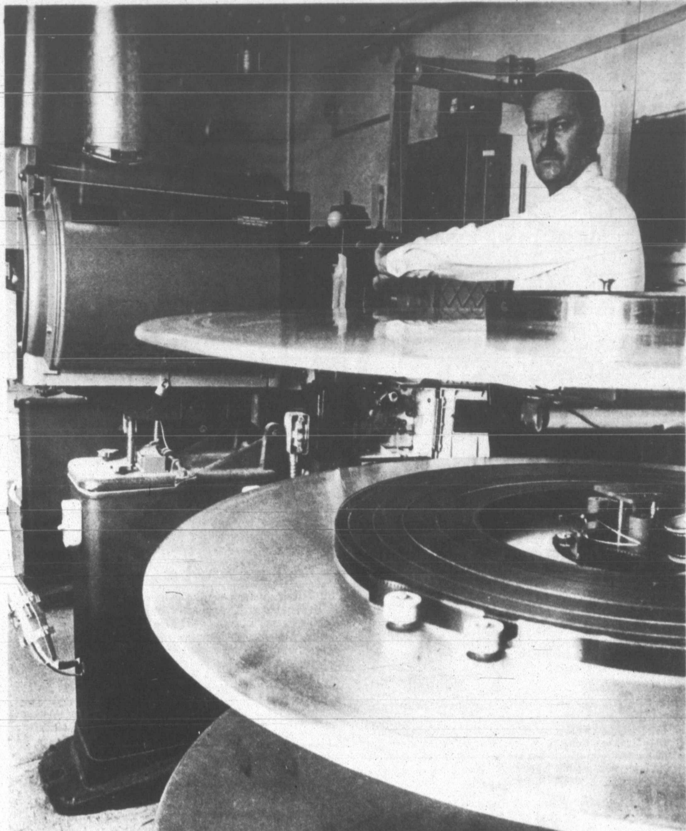
Old-fashioned reels on the movie projector at Pampa's Capri Theatre have been replaced by automated platters, explains Charlie Sartor.
