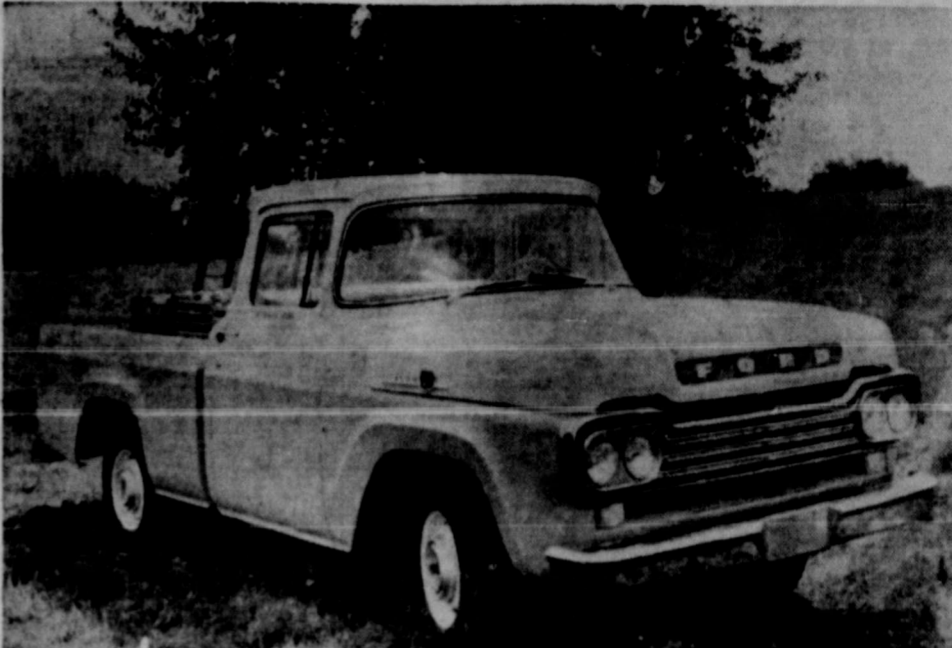
The popular F-100 pickup is one of 371 Ford truck models available in 1959. Dual headlights and a new Ford nameplate on the hood are standard features on the pickup models. With the 223 cubic inch six-cylinder engine — the most modern "six" in the industry — Ford offers greater economy in the high speed or increased load range. The pickup is available with either this Styleside body, which Ford pioneered with the 1957 models, or the Flareside body.
