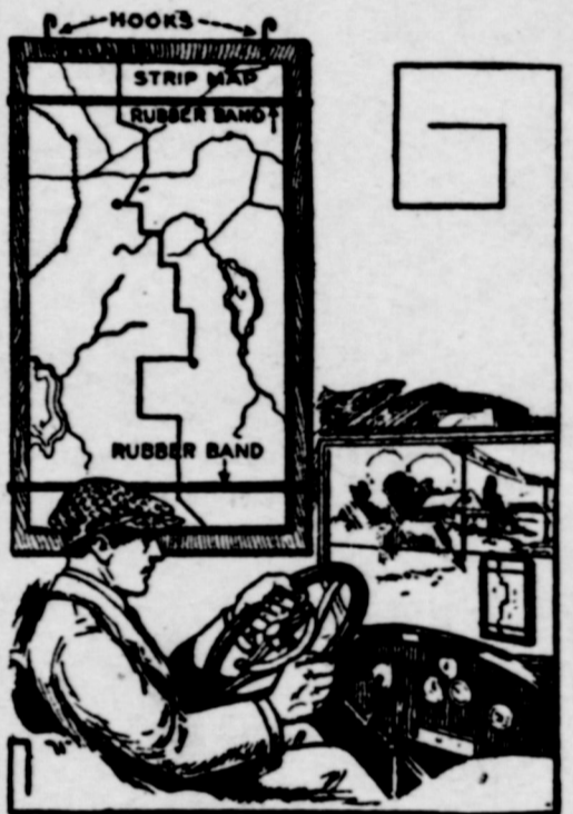
Small Road Map Mounted on Windshield in View of Driver is Convenient for Auto Tourist.
