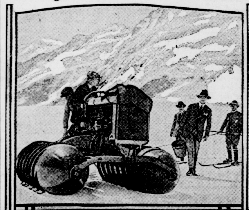
G. Scott of Detroit and J. H. Saunders of London, designers of a new style snow motor, successfully demonstrating their device at the Jungfrau-Joch, Switzerland. The motor resembles a small military tank, or tractor. It has no cogwheels, but huge drums which revolve spirally and propel the machine onward by means of threads which fasten themselves into the snow like giant screws.
