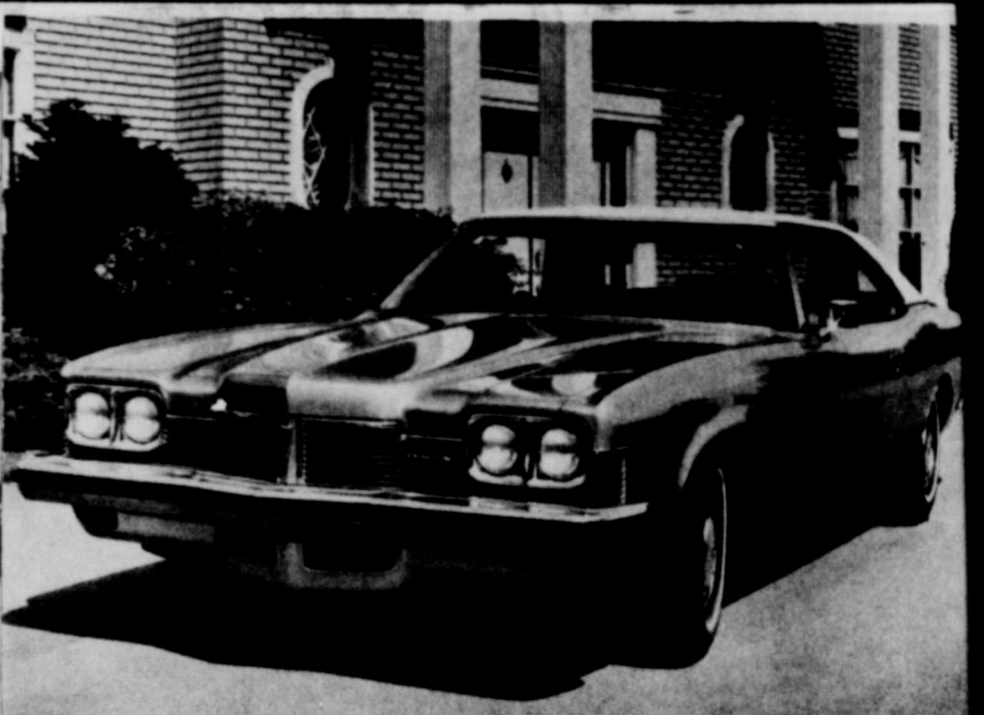
1973 CATALINA -- The popular Catalina has all-new front end sheet metal with the grille extending the full width of the front providing a strong horizontal theme. The Catalina has a front bumper system which meets the requirements of the Federal bumper standards by being completely self-restoring in a five-mile-per-hour barrier test. Bumper guards and rub strips are available.
