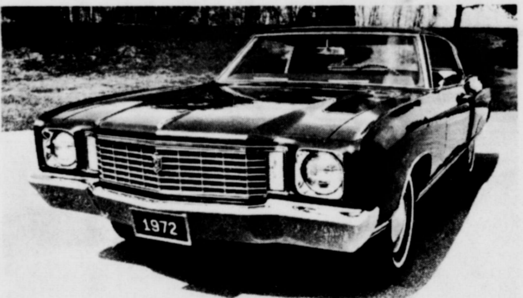
Chevrolet's personal luxury car has a new wider grille and parking lights set between the grille and Power-Beam headlights for 1972. A bright center windsplit blends into the six-foot long hood. Variable ratio power steering and power disc/drum brakes are standard. Luxury interiors, rugged body and chassis components and agile handling contribute to Monte Carlo's steadily increasing sales. All 1972 Chevrolets will be introduced Thursday, September 23.
