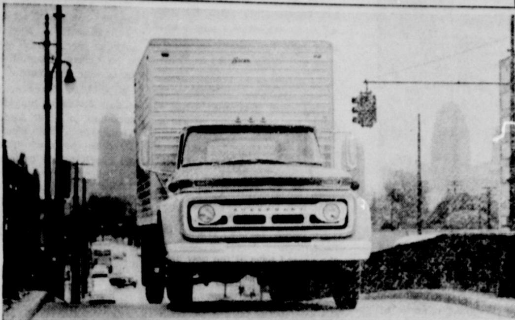
Diesel power for the first time, addition of two higher powered V8's, and lower hood lines for better road visibility highlight Chevrolet's 1962 truck line. New to most of the 198 models are directional signals as standard equipment, single
