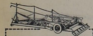
MODEL 35 —Larger, longer, more dirt capacity than Model 25. Both 25 and 35 have main frame spliced for converting in field to maneuverable dirt mover.
