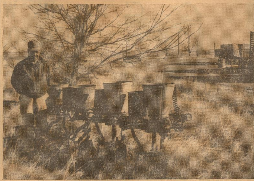
THIS HAND-MADE planter has paid off in big dividends for Carlos Calvert, Nazareth farmer. Calvert is seen standing beside the planter, which he built for his tractor. The planter is rigged to plant on 28-inch middles. It has one box for grain sorghum and one for field peas in order to inter-plant. Calvert has averaged better than 5,000 pounds of grain sorghum per acre over a 430-acre plot or a total yield of 2,360,000 pounds of grain. He has also done a good job of building up his soil in the process. (photo by Carl Leavelle)
