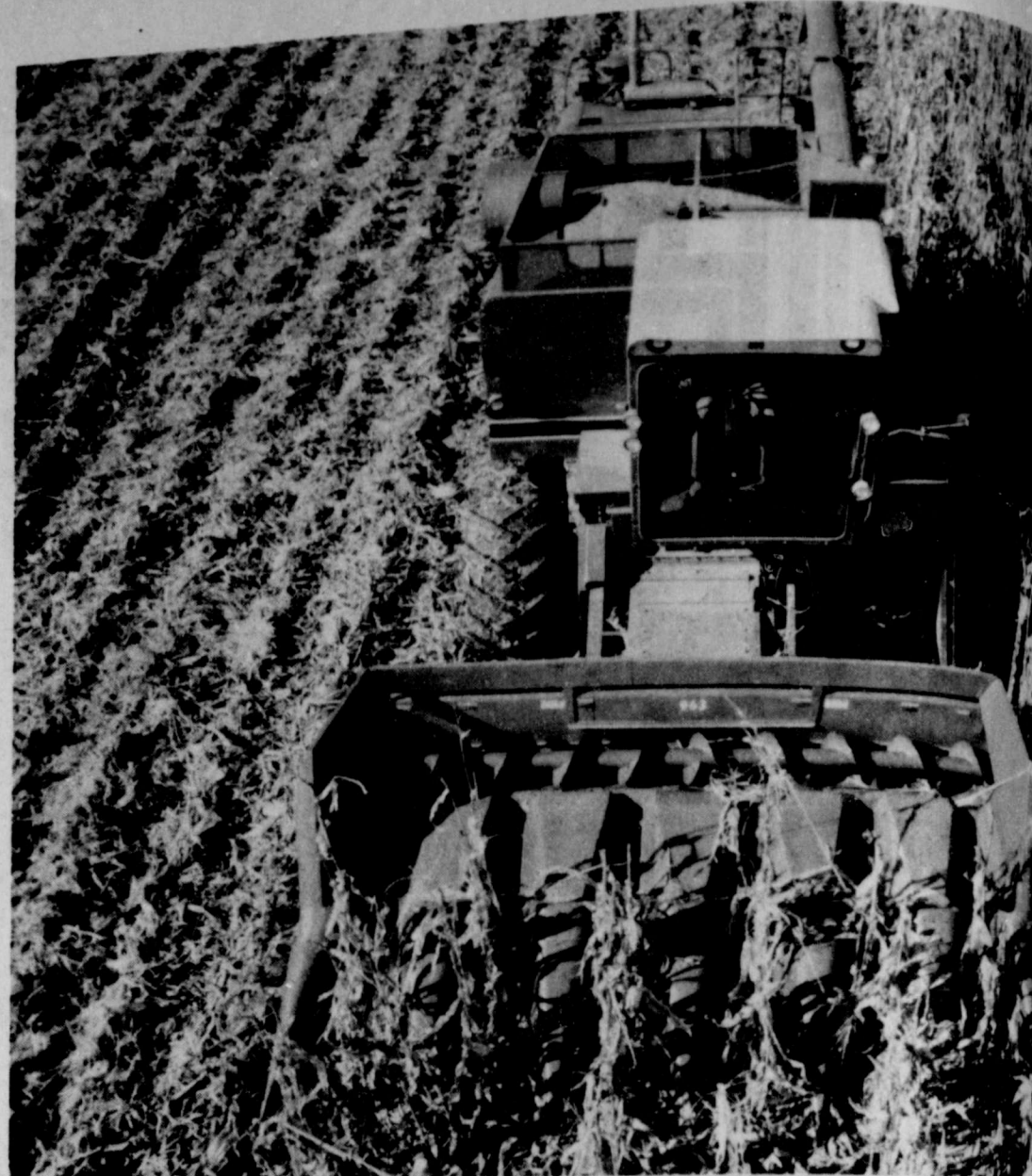
The 963 corn head is one of eight 900 Series corn heads introduced by International Harvester. The new, more efficient corn heads are 20% lighter in weight, yet stronger than previous IH models. They have longer stalk rolls that work extremely close to the ground so ears that are down or tangled.
