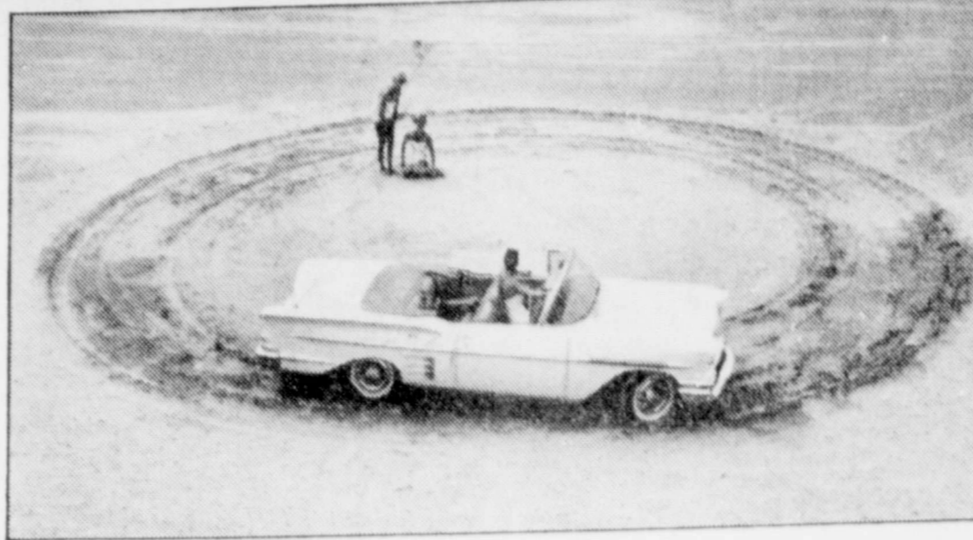
Around and around she goes and where she goes proves to be a perfect circle in the sand. Continued refinement of Chevrolet steering permits tight turns in an area 2 1/2 feet less in diameter than previous models, despite a two-and-one-half-inch increase in the car's 1955 wheelbase.
