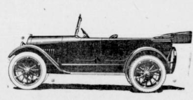
A five-passenger car of 119-inch wheelbase; light in weight with perfect balance and unusual power. Its 50-The Special horsepower demountable-head motor is most efficient and economical and is notable for its flexibility. Equipment includes cord tires, improved wind-shield with bulletshaped cowl lamps, extension tonneau lamp, outside and
