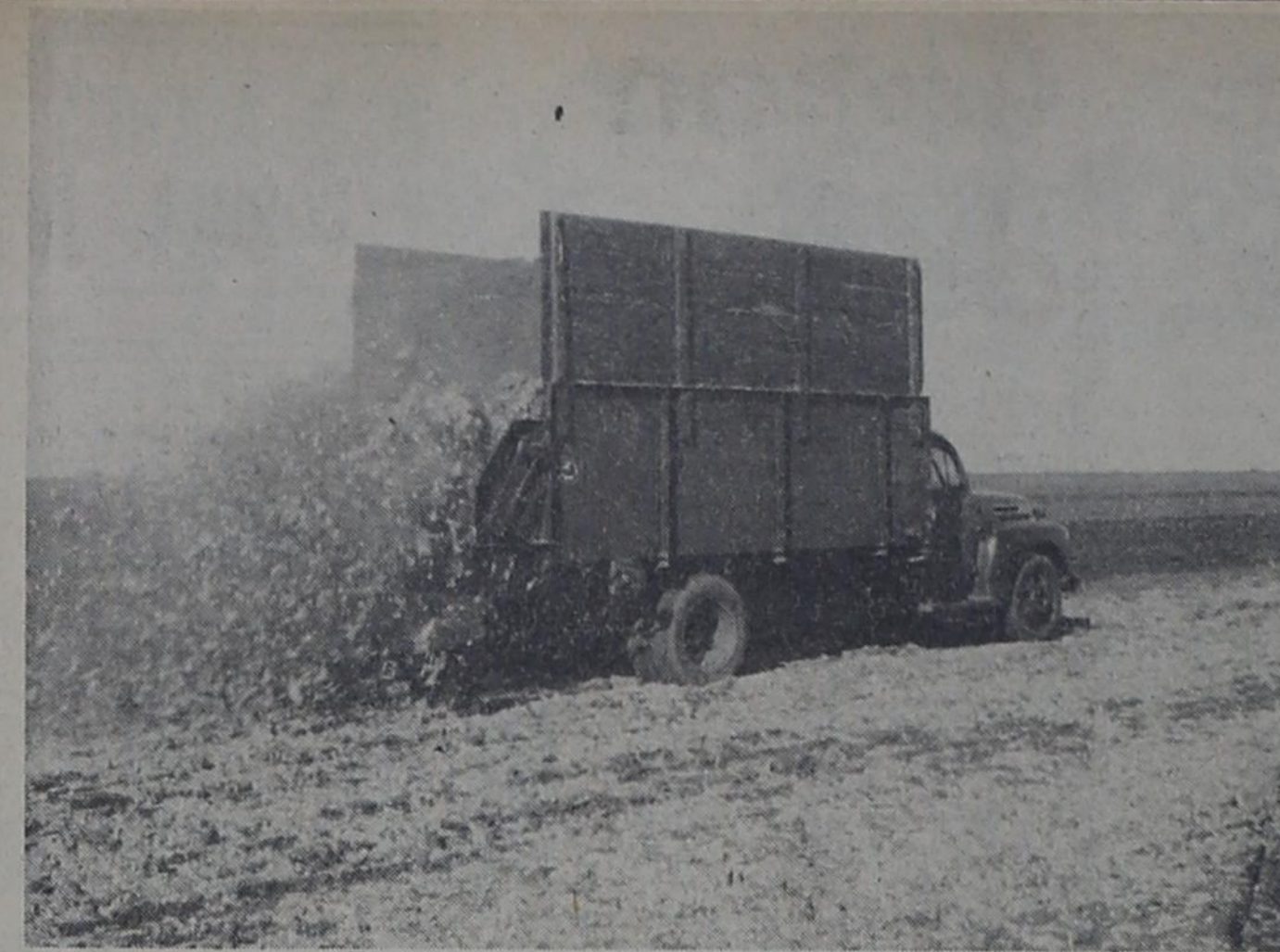
EVEN DISTRIBUTION is attained as the saw-like blades churn through the burs and scatter them over the soil as the truck rolls slowly along. The truck is emptied in a hurry this way.
