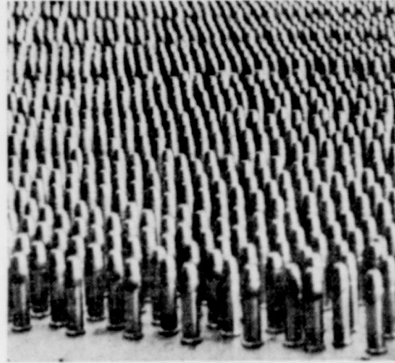
Primed, filled and capped with the lead projectile, bullets are shown here ready for packing and shipping. In a few weeks one of these bullets may whizz its way against an elusive fencepost, while its neighbor stops a jackrabbit in his tracks. If you think it's easy, try it!
