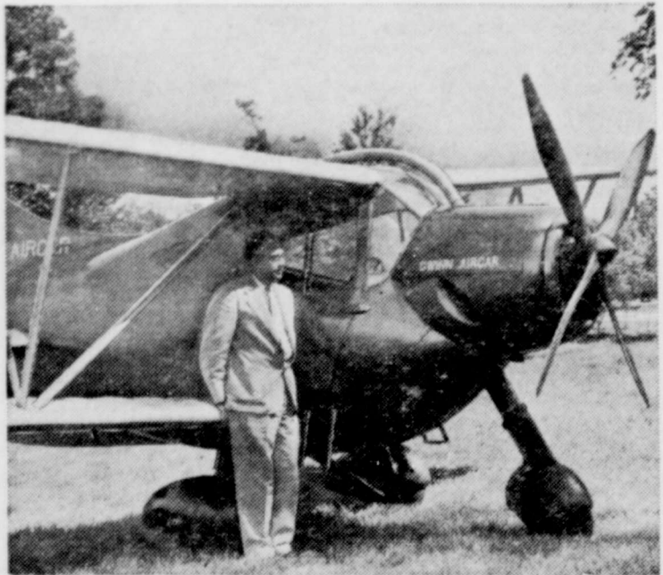
One of the "parallels" between automobile and airplane is illustrated in the tricycle landing gear which features the 1938 Gwinn Aircar.
