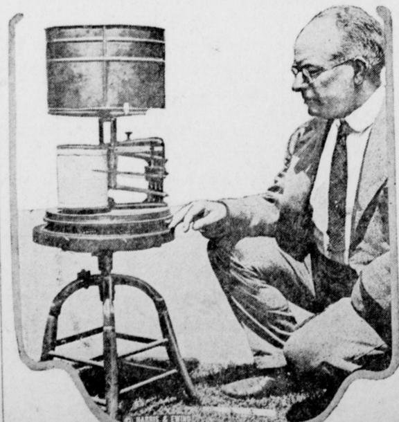
S. P. Ferguson, meteorologist of the United States weather bureau, with a gauge which he has designed to measure snow and hail as well as rain. The instrument automatically transcribes the report on a chart by means of a pen. This is the first gauge to register solid precipitation without melting the snow or hail. The old gauges required the continuous consumption of oil or gas for this purpose.
